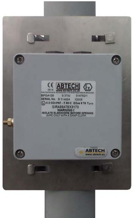
Each enclosure comes pre-drilled with four M20 tapped cable entries and is supplied with certified blanking plugs. The BPGA range of enclosures are ATEX and IECEx certified Ex'e' and are suitable for use in Category 2/Zone 1 & 21 and Category 3/Zone 2 & 22 areas according to EN 60079-14.
