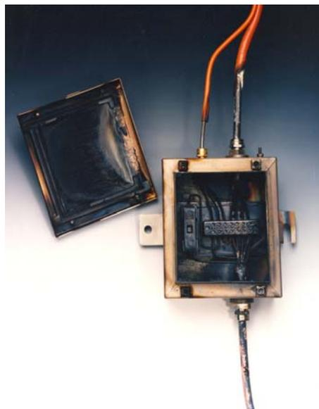
On the successful conclusion of this test, which is designated “fire-alone” BS6387 ‘C’, the next test is to mount the sample (still powered-up) on a flat vertical surface and to apply flame at a temperature of 950°C (1742°F) (by means of a flame gun) whilst at the same time striking the board on which the sample is mounted with a 25mm (1”) diameter iron bar every 30 seconds for a period of 15 minutes. This is designated the “impact test” BS6387 ‘Z’.
