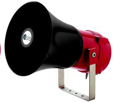
BExDS120D & BExDS120E Flameproof & Dust ignition proof sounders Zones 1, 2, 21 & 22 ⊕ II 2G/D EEx d IIC T4 T100°C ⊕ II 2G/D EEx de IIC T4 T100°C
